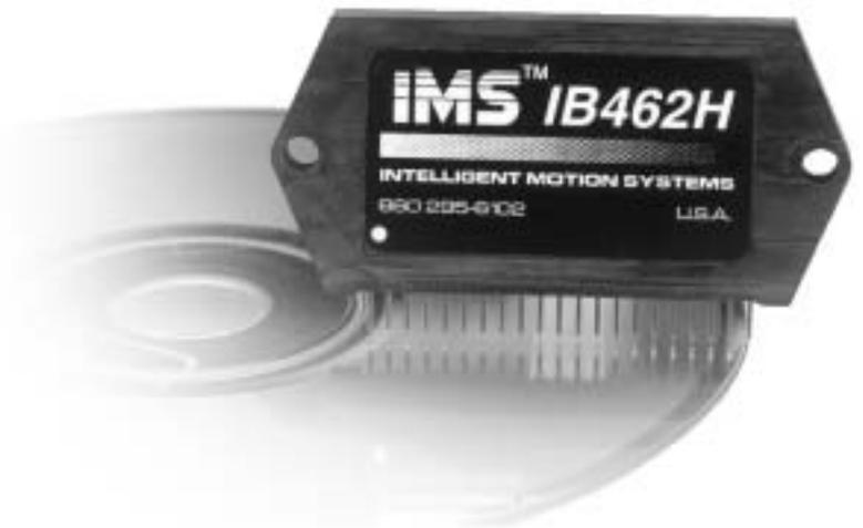
is preferred. The INT-462 is much more than a simple pluggable interface. It adds a dynamic array of features to the IB462H that are found only on larger more expensive drives. Features such as a +5 VDC switching power supply, +5 to +40 VDC opto-isolated inputs which are internally limited to 8mA, automatic current reduction, over current and short circuit protection, input capacitor, and fault and power LEDs. Wiring is done through a 15 pin removable screw terminal.
