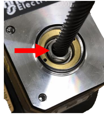
Figure 2: External Linear Actuator with New Insert Design
