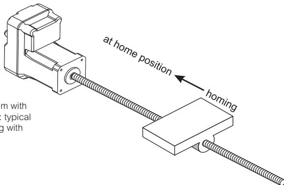
Closed loop system with absolute encoder: typical sensorless homing with linear motion axis.
