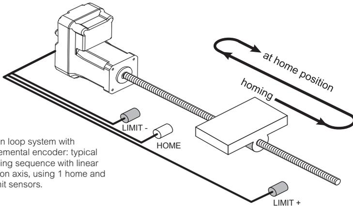
Open loop system with incremental encoder: typical homing sequence with linear motion axis, using 1 home and 2 limit sensors.
